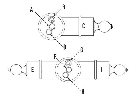
Hoses are attached to faucet body as shown in diagram.
