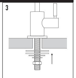
Place faucet handle in desired position. Fasten the faucet from under the countertop, sliding large rubber washer, then metal washer, then smaller rubber washer, then 5/8" diameter serrated lock washer on the faucet stem, and secure with the lock nut so the faucet does not move/spin.
