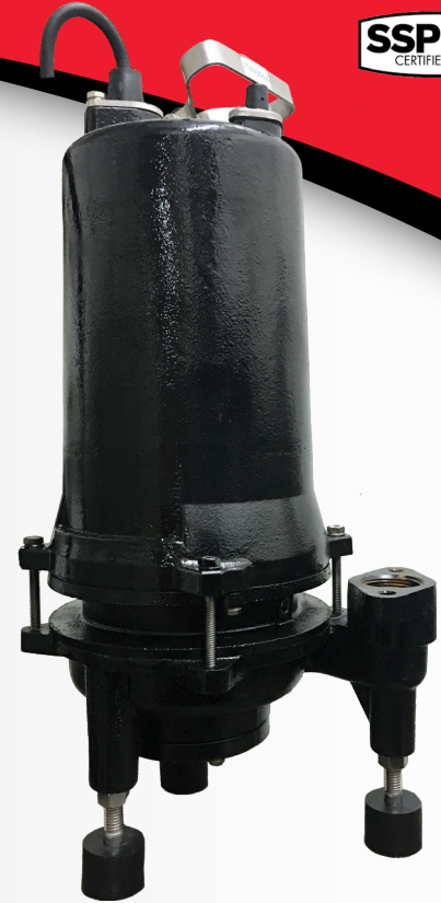
2 HP grinder pumps that have a 1 1/4" or 2" optional vertical discharge that handles up to 3" solids
